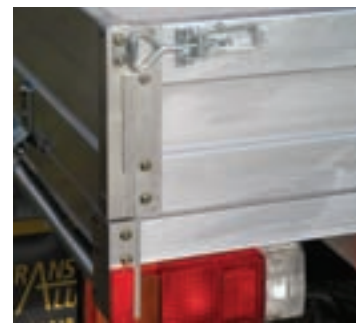
Heavy duty zinc plated hinges & corner fasteners
