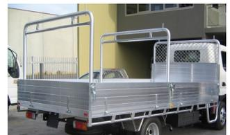
Transalloy has designed a rear rack to suit each of our tray bodies—all of which have been engineer tested and designed to comply with RTA standards.
